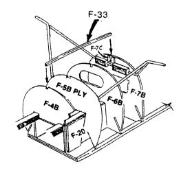
[L] 13. Glue [1] F-33 FRONT BOTTOM STRINGER (5/16 sq. x 9) from F-4B PLY (1/8 Die Cut) thru F-7B PLY (1/8 Die Cut).
